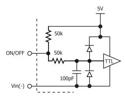
Figure B: Internal ON/OFF pin circuitry
