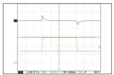
Figure 6: Output voltage response to step-change in input voltage (1000 V/ms), at Max. load current.Load cap: 1 µF ceramic cap. Ch 1: Vout, Ch 2: Vin.
