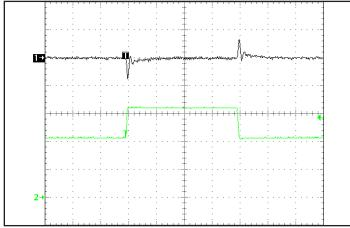
Figure 5: Output voltage response to step-change in load current (50 % -75 %-50 % of Iout(max);  $dI/dt = 0.05 A/\mu s$ ). Load cap: 15  $\mu F$  tantalum cap and 1  $\mu F$ ceramic cap. Ch 1: Vout, Ch 2: Iout.
