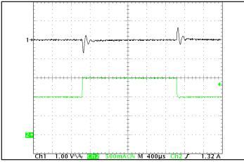
Figure 5: Output voltage response to step-change in load current (50 % -75 %-50 % of Iout(max);  $dI/dt = 0.05 A/\mu s$ ). Load cap: 1  $\mu F$  ceramic cap. Ch 1: Vout, Ch 2: Iout.
